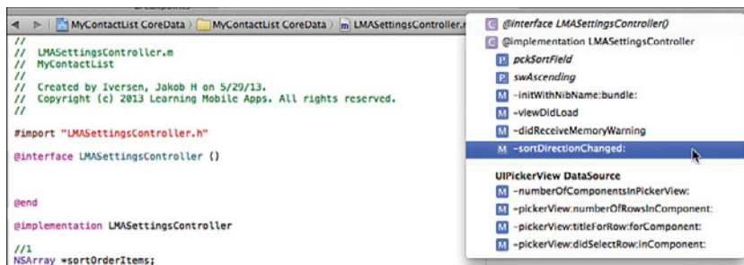
Figure 11.12 Drop-down menu on the right showing the result of #pragma mark in the code.
